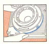
For flash work the fully automatic mechanism is disconnected. Turn the milled setting disk anticlockwise until the lightning symbol appears against the triangular mark and the flash contact becomes visible—the V lever is then blocked and must not be pressed when taking flash photographs! There is now a choice of apertures from f. 3.9 to 22 which have to be set by hand and are visible in a small window on the shutter.
