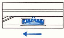
Then operate the rapid transport lever as already described, press the V lever and release the shutter. Repeat this process twice more and your camera is then ready for the first exposure. The film counter indicates the number of exposures still left on the film.
